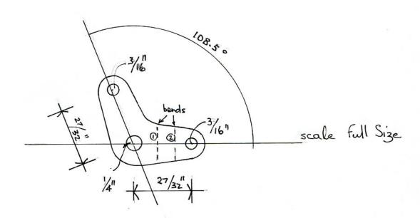
Secure the larger part of the plate in the vice up to the bend point 1. Then bend it away from you to about 20 degrees. Finally put the tip in the vice up to bend point 2 and tap the plate forward by a similar amount to bring the tail parallel to the main area. You will need a  $\frac{1}{2}$ " x  $\frac{3}{16}$ " round-head steel rivet to secure it to the original pawl. Sorry not to be able to supply the parts but my supply is now exhausted.
