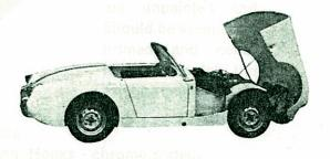
frontal area the Monza bonnet is very much lighter than the Mark I assembly or Mark II bonnet and wings. Another advantage is engine accessibility which
